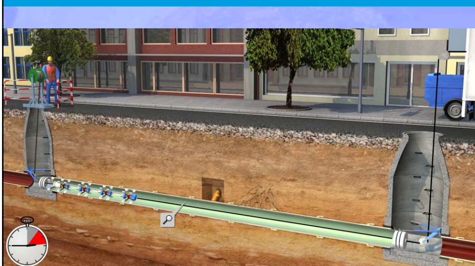
CIPP - Preparation for curing process
