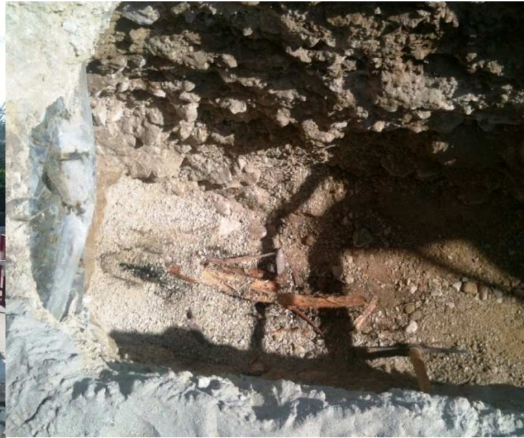
Roots with Ø 90 mm in the old pipe
